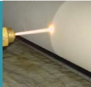
HVOF spraying of rollers for printing.
