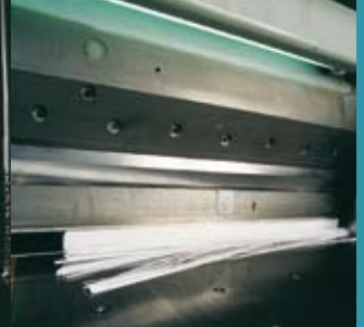
Extremely hard wolfram carbide surfacing keeps cutter blades sharp in the paper industry.
