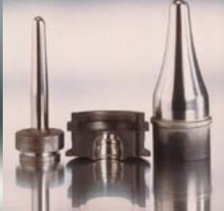
Efficiently applied high wear resistant surface on bottle plunger and neck rings.
